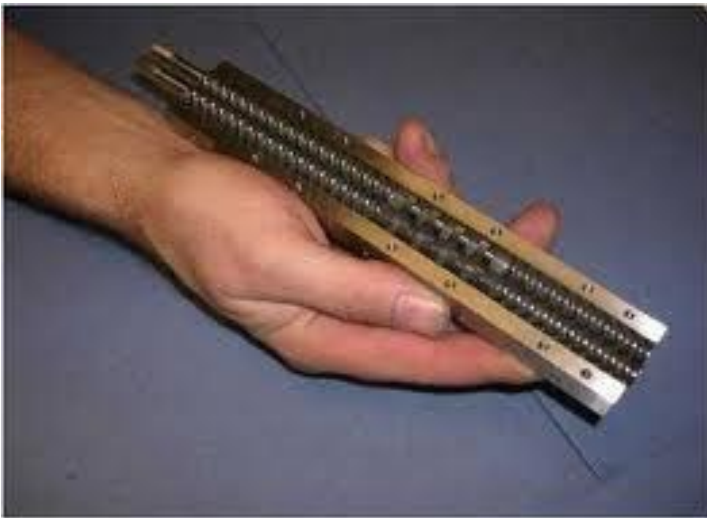
Lab scale twin screw extruder for both mixing and extrusion
